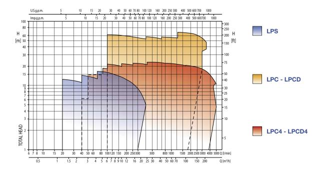
The in-line centrifugal pumps, both in the steel and cast iron version, for applications related to circulation with certain advantages. Their constructive configuration with suction and discharge on the same axis allows easy and simple installation and optimises their positioning.
